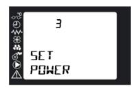
To change the operating output, press Key **5** on the main page to immediately open the screen where you can use Keys **1** and **2** to select from the five settable output settings. After selecting the required output level, press Key **3** to return to the main page.
