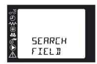
If the channel set in the electronic card does not match the one set on the remote control, the SEARCH FIELD message will remain on the display. If, however, the channel is correct, message UNIT LOADED X will be displayed.
